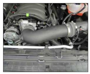
7. Install the K&N<sup>®</sup> intake tube into the coupler at the filter housing and then into the coupler at the throttle body, adjust the tube for best fit and then secure with the provided hose clamps.
