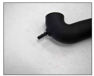
5. Install the provided quick disconnect fitting into the K&N<sup>®</sup> intake tube as shown.
